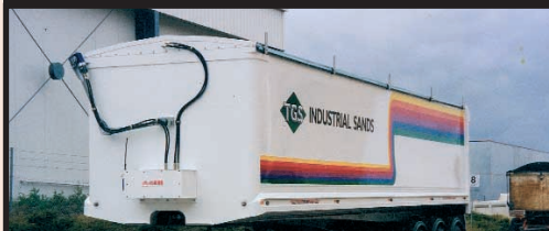
Electric and hydraulic kits for Roll Over tarps
