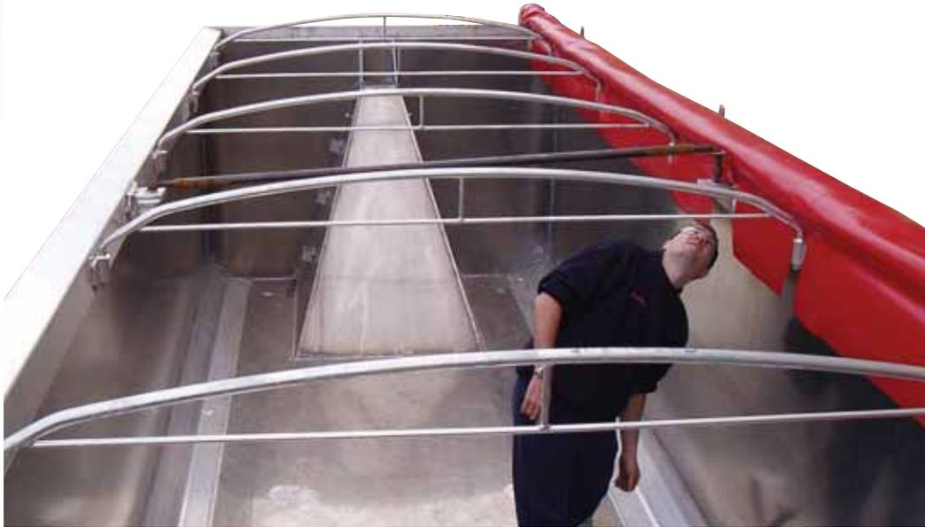
roll over tarp with its tarp bows and centre bar is not suitable for quarry work, where vehicles are loaded by wheel loaders and excavators. And a mesh wind-out tarp is not suitable for grain and fertilizer, because it has to be waterproof."
